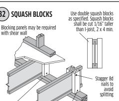
Toe-nail 8d nail to plate
