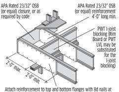
6" oc. Stagger nails from both sides in C3 to avoid splitting.
