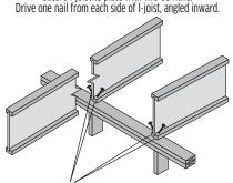
Place nail 1-1/2" min. from end of I-joist. If nails are close to edge of plate, drive at an angle to reduce splitting.
