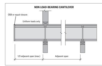
LPI blocking or other lateral support required at ends of I-Joist
