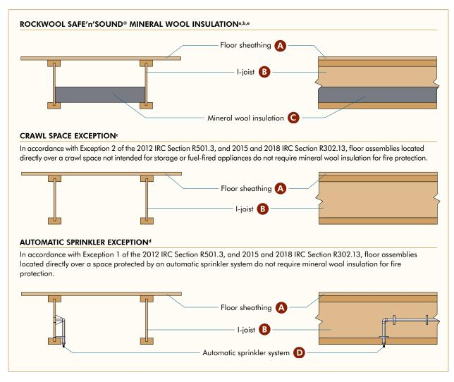
A Floor sheathing: Materials and installation in accordance with 2012, 2015 and 2018 IRC Section R503.
