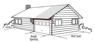
This table provides PWLVL header sizes for the support of roof trusses over various rough openings. A 2-foot maximum roof overhang is assumed.
